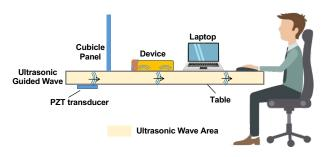
Fig. 1: *SurfingAttack* leverages ultrasonic guided wave in the table generated by an ultrasonic transducer concealed beneath the table.
