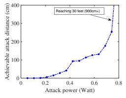
Fig. 14: Relationship between attack power and distance.
